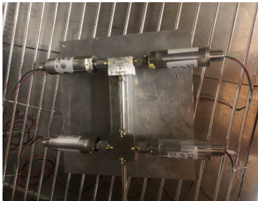
Four sensors (S1,S2,S3,S4) pressure cycled with hydrogen gas
