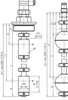
\* Immersion depth at densityc 1:  $VA52 = 36 \pm 2 \text{ mm}$  $BN30 = 20 \pm 2 mm$ VA44 = 36 ±2mm (52 mm high) VA80 = 36 ±2 mm (80 mm high)
